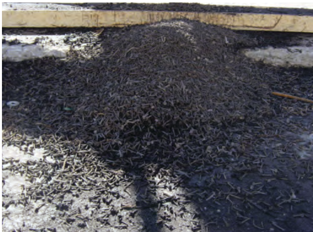
Figure 7-5. Nails Taken from PCAS Material During Processing.
