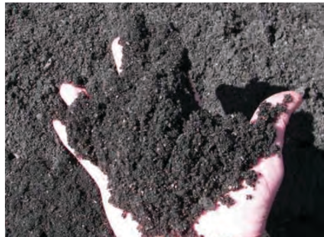
Figure 7-6. Processed RAS Should Have the Consistency and Appearance of Coffee Grounds (Surti, 2012).
