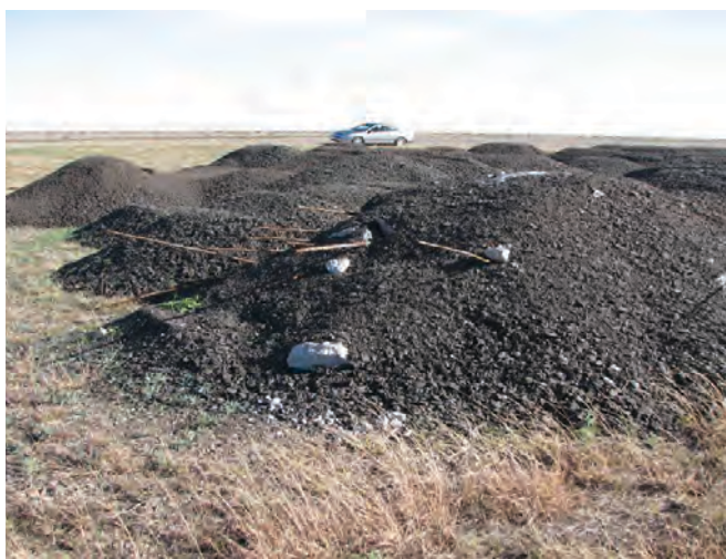
Figure 7-1. RAP Stockpiles. (a) Contaminated Stockpile (left); (b) Well-Maintained Stockpile (right).
